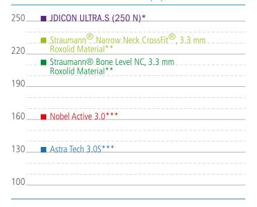
Fatigue strength is the maximum force an implant / abutment structure can survive for at least five million cycles. JDIcon Ultra.S has been tested according to ISO 14801 that is accepted by many regulatory agencies including FDA and Notified Bodies (CE).
